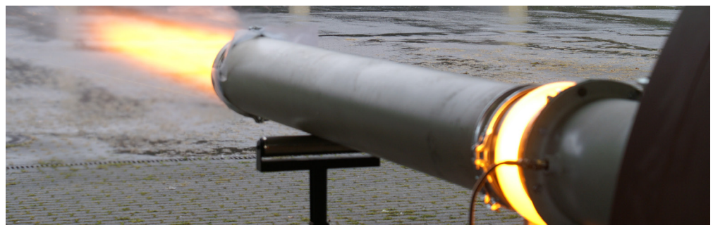
Fig. 5 - Jacob pipe and flexible connector system during the explosion
