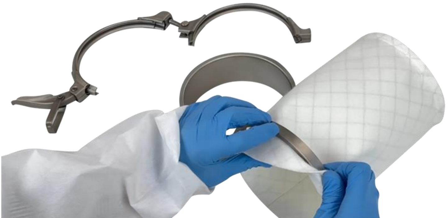
Fold the disposable filter bag / breather bag around the Jacob flange.
